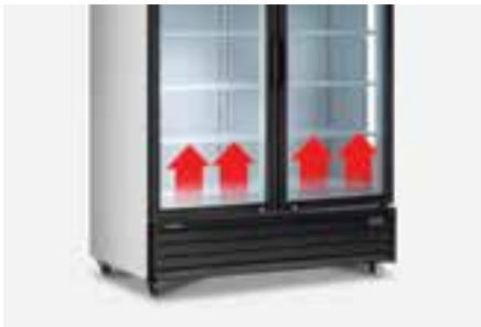
Hot Air Blowing To ensure that display items stay clearly visible, hot air flows from the compressor to the showcase door, preventing condensation from forming on the glass.
