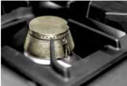
Gas Safety Device Each burner is fitted with a thermocouple safety sensor that automatically shuts off the gas flow as soon as the burner flame is extinguished.
