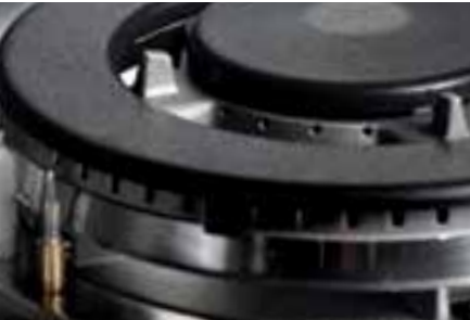
Gas Safety Technology Ensures burner and oven safety, as the thermocouple sensor shuts off the gas flow as soon as the flame is extinguished.
